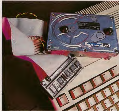
The Quantum hard drive (seen here with an ICD Prima internal unit) doesn't have a fan of any sort.
